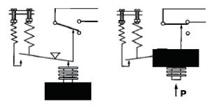
A flexible sensing element actuates a microswitch by means of a lever. The set point is adjusted by means of a compressible spring installed in opposition.
