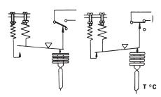
Set point and reset point must be between 10% and 90% of the selected scale.
